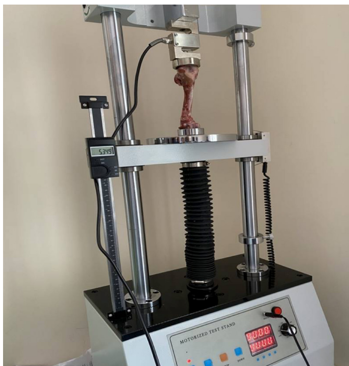
Figure 2. Application of axial force to the lamb bone using the Geratech SH 5000 testing system.
